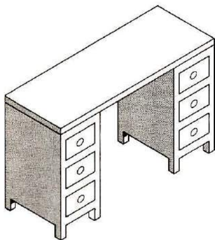
Fig. 1. A place to start: An old table-top, or door, or plywood top, placed across a pair of pedestals from a cast-off desk, some old furniture, or even constructed from scratch. It'll hold two or three pieces of equipment plus a key or microphone, with storage for paper, log books, and those spare parts and tools you'll find essential to maintain your station.
